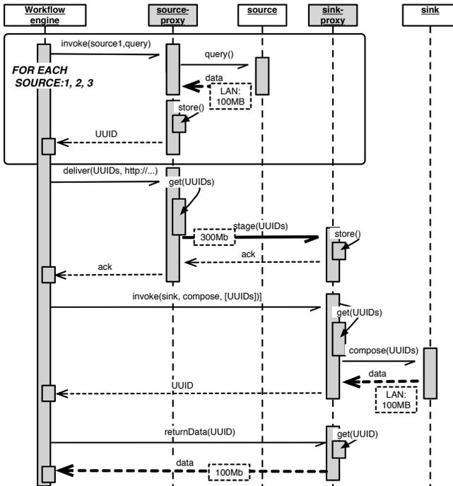
Fig. 3. UML Sequence diagram—Circulate fan-in.
