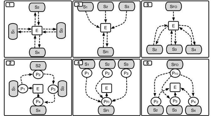
Fig. 5. Experiment setup used for the analytical model and the pattern-based performance analysis. Data flow in the sequential (first column), fan-in (second column) and fan-out (third column) patterns for the centralised architecture using standard services (1,3,5) and the Circulate architecture (2,4,6). Control flow messages are omitted. This example shows 4 services, each proxy is deployed on the same server as the service it is invoking.
