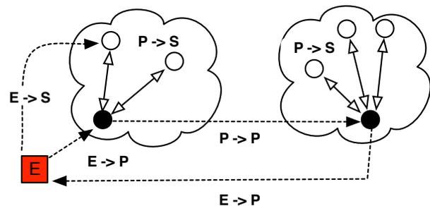
Fig. 1. Actors and interactions of the Circulate architecture. Web services are represented by hollow circles, proxies by solid circles, the workflow engine as a square, dashed lines are WAN hops, solid lines LAN hops.
