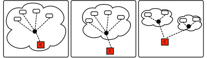
Fig. 6. Configurations from left to right: local LAN, remote LAN, Internet-scale. Services, proxies and the workflow engine are always deployed on separate machines.
