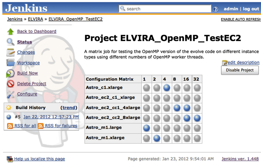
Figure 3 A project configured in Jenkins to run a set of jobs defined through a matrix of parameters (here, the worker node and the number of threads to use, cf. Table 3). A filter condition has been applied to make this a sparse matrix.
